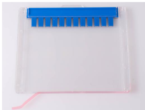
Figure1. Remove the pink tape at the bottom of the gel plate.
