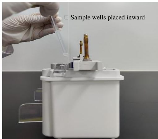
Figure 3. Insert the gel plate into the gel electrophoresis apparatus.
